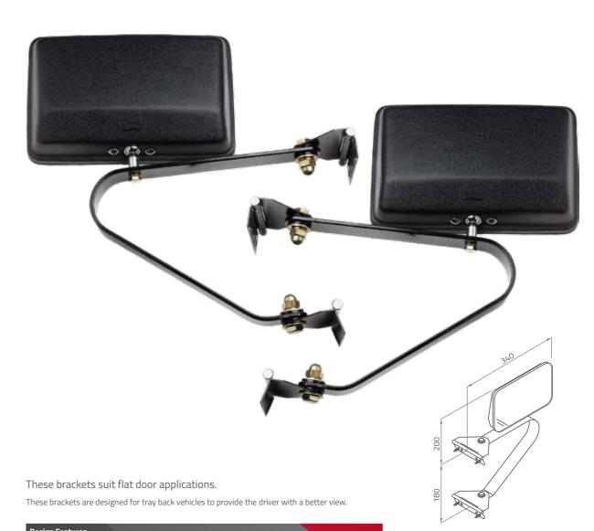
Galvanised powder coated steel swing arm and mounting bracket
