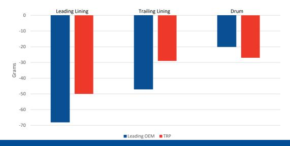
The above graph shows total weight loss of the linings and drum after the FMVSS 121 test has been completed. The smaller the bar the better the result. The leading OEM brake shoe manufacturer results have also been included. The comparison shows that TRP® linings outlast the OEM equivalent by up to 30% and deliver a better return on investment.
